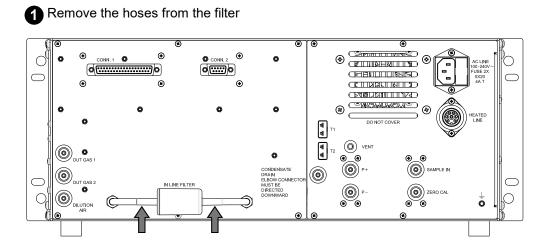
2 Replace the dust filter with a new one. See chapter "Spare parts"
