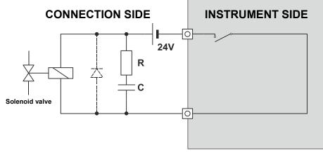
Figure: Sparks suppression on a relay contact
