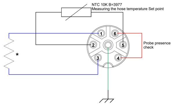
\*: Heater 110V 195W for 3 meters of hose (65W / m). It is possible to power up to 500W corresponding to 8 meters of hose.
