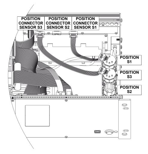
The upgrading of the number of sensors can be easily done by the user by performing the following directions:
