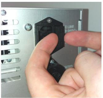
2 Extract the fuses, using a screwdriver, paying attention not to damage the fuse holder and/or the fuses themselves.
