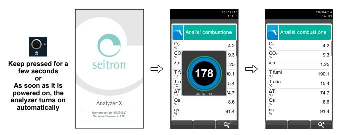
• The instrument then performs automatically the emission analysis according to the configuration made.
