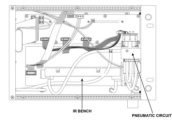
An infrared bench for the detection of gases based on (NDIR) infrared spectroscopy can be installed on **CHEMIST 900 RACK**.
