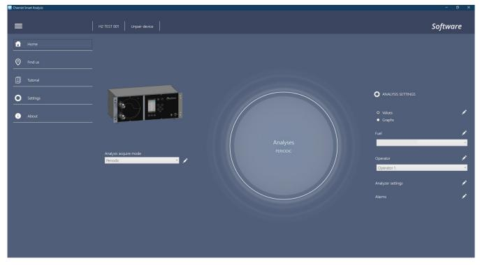
By clicking on the symbol "**Start recording**", the emission analysis begins according to the settings made; the data of the emission analysis are saved in a csv. file.
