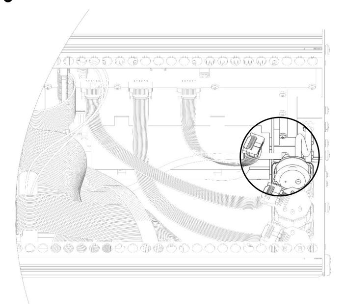
6 Fit the new sensor again taking care the electric connection is turned to the outside the instrument, not the inside (See point 4).
