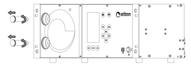
3 Clean the cover inside by using compressed air, soap and water or ultrasonic cleaner (do not use solvents or thinners as the case/container is made of PVC plastic material).
