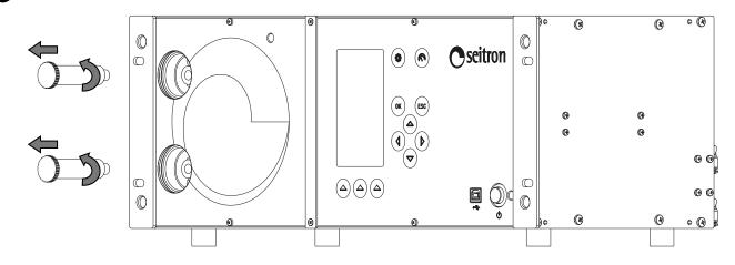
**3** Replace the paper filter with the HDPE filter and screw it back on its seat.
